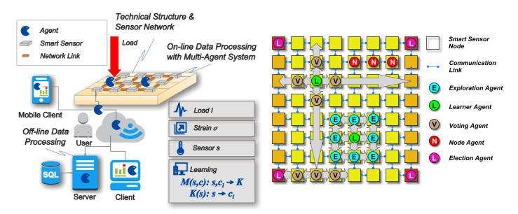
**Figure 5.** (Left) Technical structure equipped with a sensor network and connected to Intra- and Internet environments (Right) Logical network view and deployment with multiple agents instantiated from different behaviour classes.
